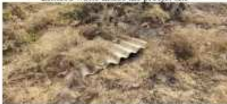
ACM left near the Overhead Water Tank
